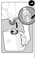
Attach the floating cable to the power supply.
